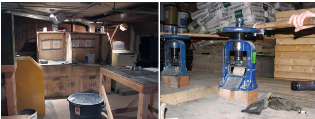
Preparation facility inside warehouse Core cutting facility with manual splitter
